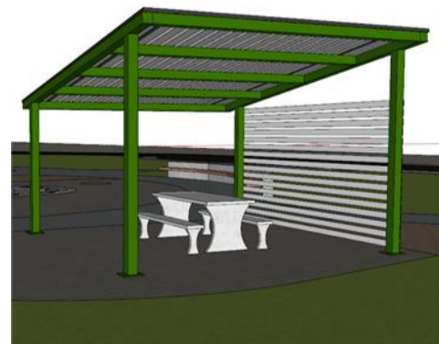
COLORBOND SKILLION ROOF TO POWDER COATED ALUMINIUM STRUCTURE. OVERALL STRUCTURE SIZE 5700x4600mm. WHITE HORIZONTAL SLAT TO 2450mm HIGH TO 3 SIDES OF STRUCTURE.
