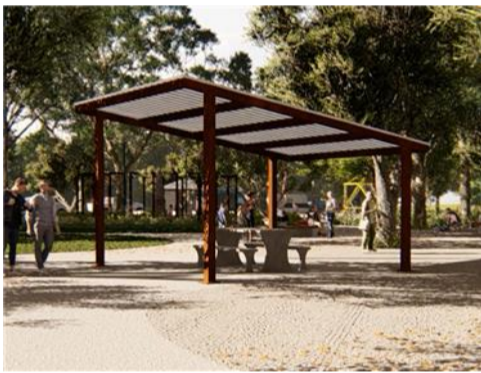
COLORBOND SKILLION ROOF TO POWDER COATED ALUMINIUM STRUCTURE. OVERALL STRUCTURE SIZE 5700x4700mm. WHITE HORIZONTAL SLAT TO 2450mm HIGH TO 3 SIDES OF STRUCTURE.
