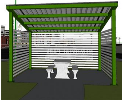
COLORBOND SKILLION ROOF TO POWDER COATED ALUMINIUM STRUCTURE. OVERALL STRUCTURE SIZE 5700x4700mm. WHITE HORIZONTAL SLAT TO 2450mm HIGH TO 3 SIDES OF STRUCTURE.
