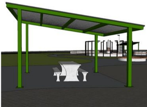
COLORBOND SKILLION ROOF TO POWDER COATED ALUMINIUM STRUCTURE. OVERALL STRUCTURE SIZE 5700x4600mm. WHITE HORIZONTAL SLAT TO 2450mm HIGH TO 3 SIDES OF STRUCTURE.
